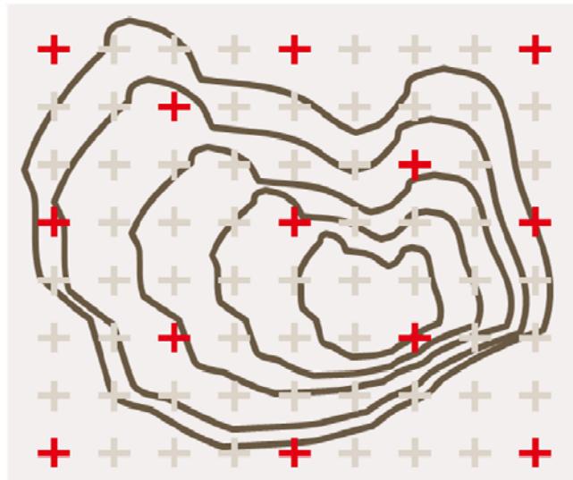
Figure 1. Typical HybridGravity™ survey scheme. All points are occupied with a relative gravity meter, and the red points are occupied with an absolute gravity meter. In this example, there are 72 total stations, 13 of which are occupied with the absolute instrument.
