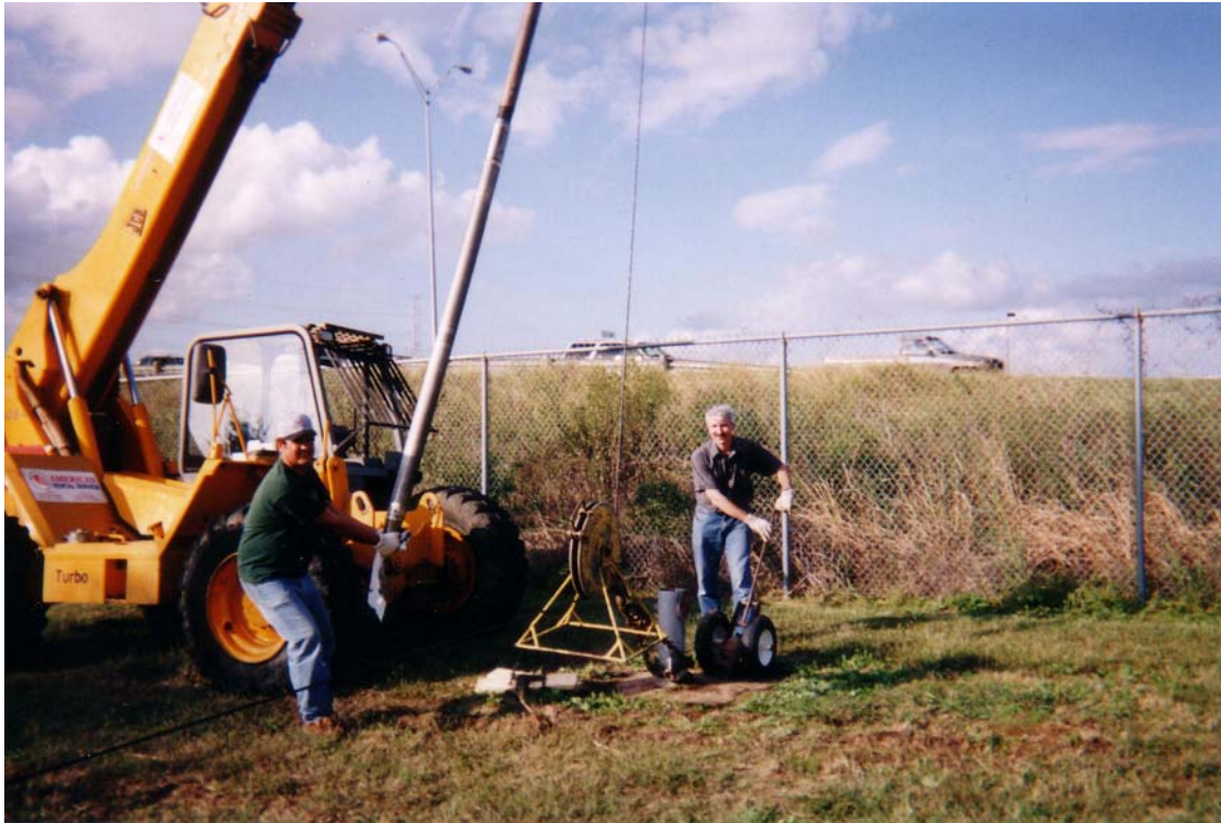
Figure 2 Deploying the BHGM in the test well
