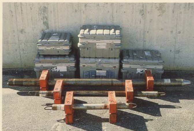
Figure 6 BHGM support equipment
