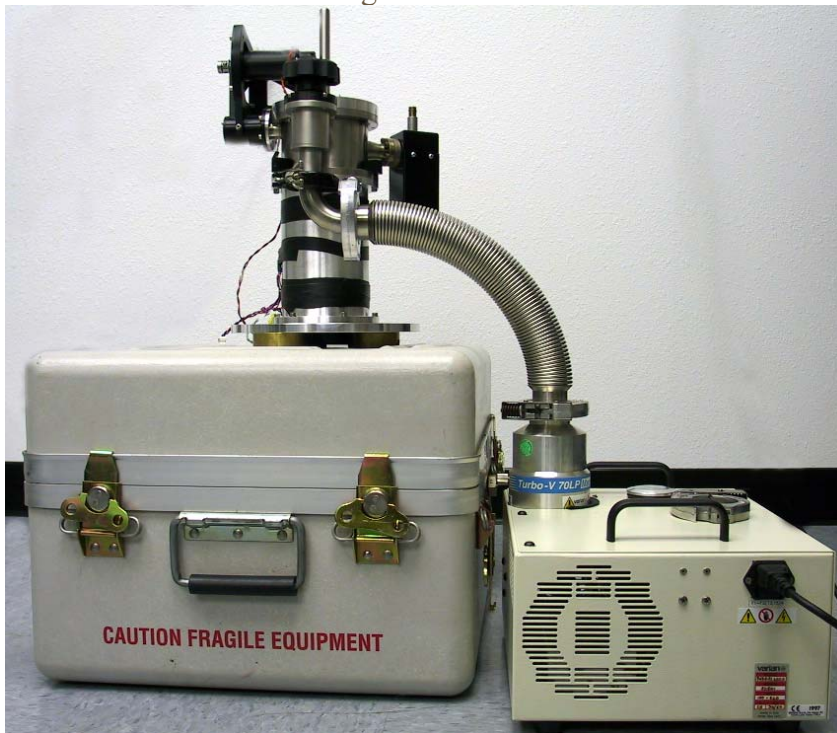
Figure 13. Turbo pump connected to dropping chamber. Note the minimum stress in the hose.
