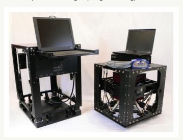
Shown above are the older TAGS on the left (without safety cages installed), and TAGS-6 on the right (no safety cages necessary).
