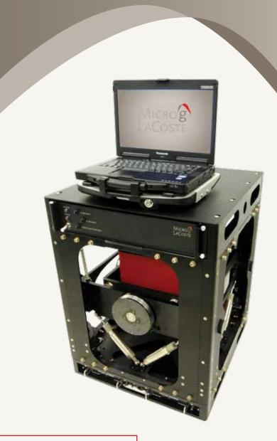
The latest in a line of Marine Gravity Meters going back over 50 years. The MGS-6: Smaller, lighter, and over 100X more quiet than its predecessor.
