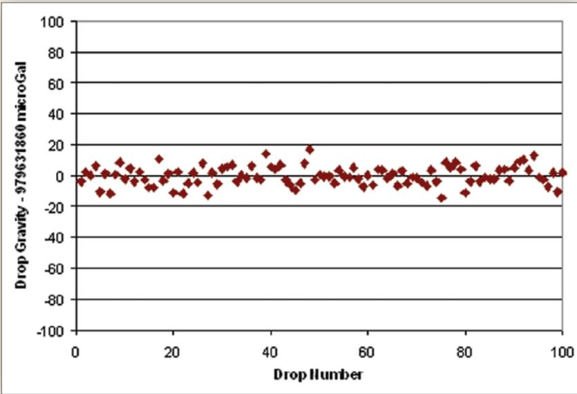
Shown above are individual measurements in a laboratory setting. The standard deviation between drops is better than 6  $\mu\text{Gal}$ . Note that the measured absolute gravity value, in this case 979 631 858  $\mu\text{Gal}$ , is computed and reported in real time.
