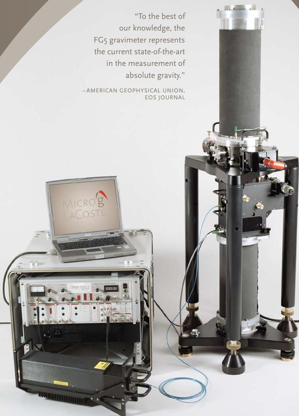
Since its introduction in 1992, the FG5 has become the industry standard in absolute gravity instrumentation. Based directly on international standards of time and distance, the FG5 provides unparalleled accuracy and precision. Whether applied in geophysical research, environmental monitoring, or laboratory metrology, the FG5 is still the highest quality, most versatile absolute gravimeter available today.
