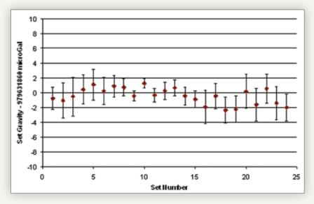
Shown above are the results of a 24-hour site occupation (24 sets of 100 drops each). The set scatter is on the order of 1  $\mu$ Gal, indicating sub- $\mu$ Gal measurement precision.
