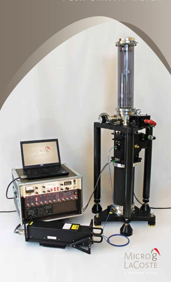
ince its introduction in 1992, the FG5 has become the industry standard in absolute gravity instrumentation, and now Micro-g LaCoste is proud to produce the latest version: the FG5X. Based directly on international standards of time and distance, the FG5X provides unparalleled accuracy and precision. Whether applied in geophysical research, environmental monitoring, or laboratory metrology, the FG5X is still the highest quality, most versatile absolute gravimeter available today.
