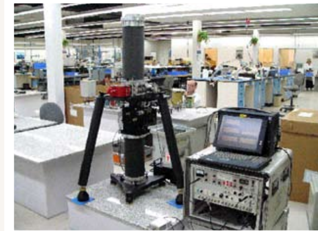
FIGURE 3 FG5 establishing an absolute station in a laboratory in Canada
